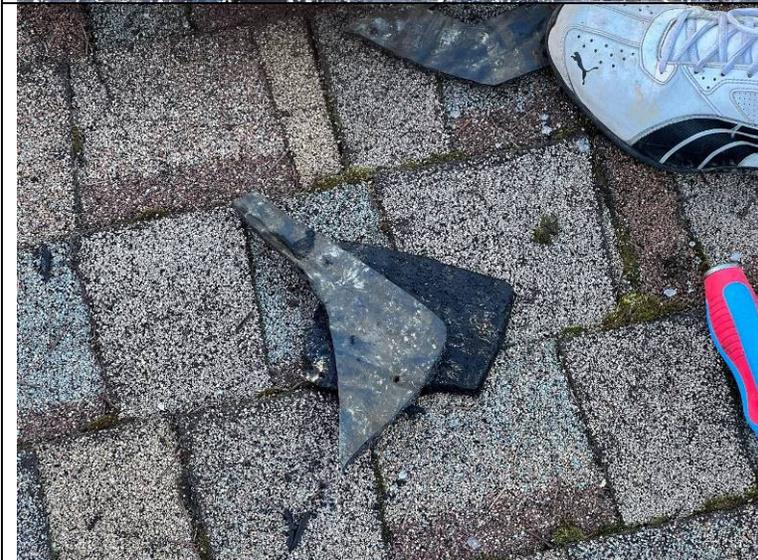
Photograph 15: Asphaltic membrane with a polyethylene surfacing.
